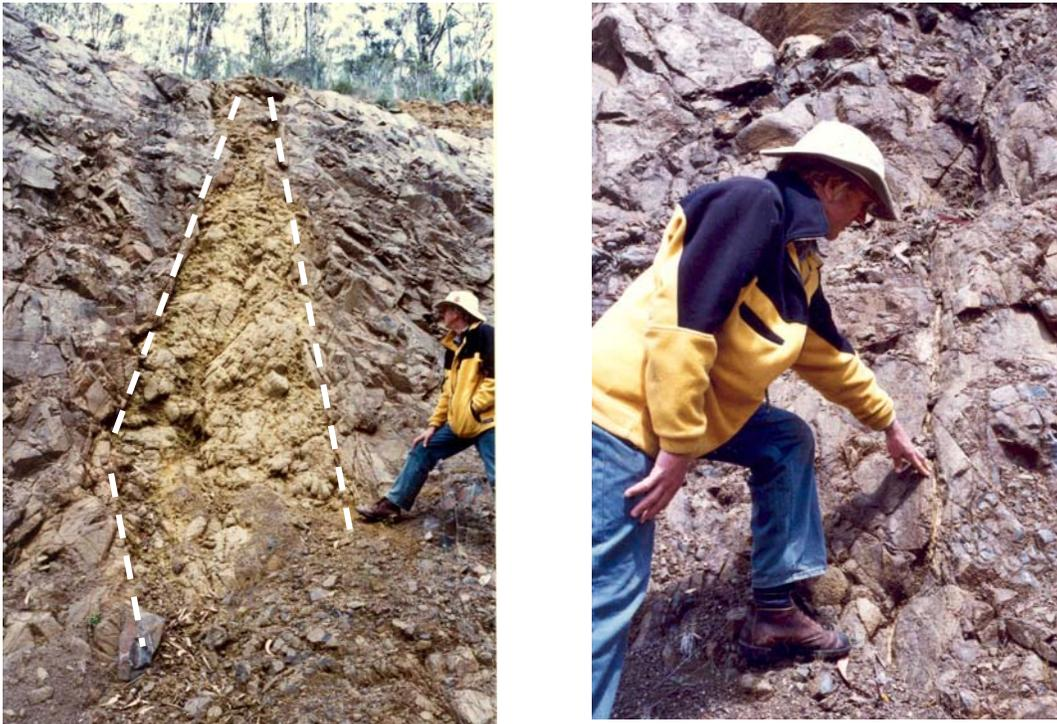
**Figure 2.** Weathered fracture zones in dolerite. These weathered fracture zones are likely to be important infiltration pathways for moisture. The zones range from >1 m to 1 cm wide.
