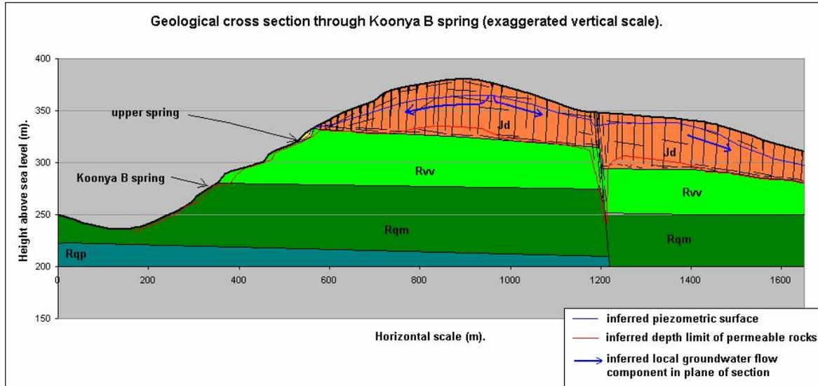
**Figure 3.** West to east (left to right) geological cross-section through the Koonya B sampling site, the sandstone cliff (marked as “upper spring”) and the inferred aquifer in dolerite. Note the fault line which may direct some drainage in a northerly direction. Note also the dolerite contact with the sedimentary beds below is inclined eastwards, but that because of the likely convex shape of the aquifer surface, some subsurface water flow is westwards. From Forsyth (2003, figure 12).
