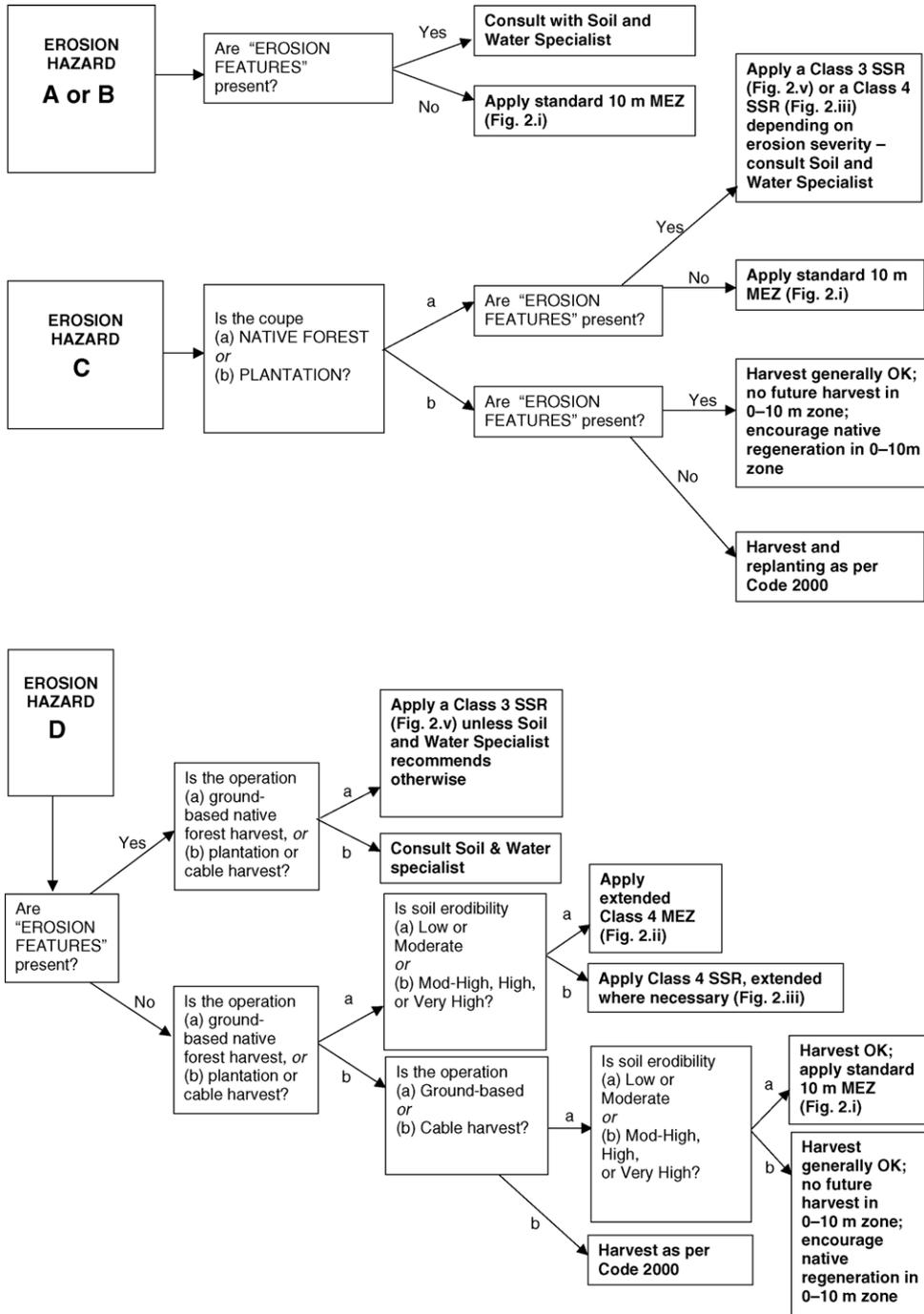
Fig. 4. Flow diagrams for keying out prescriptions for Class 4 streams.
