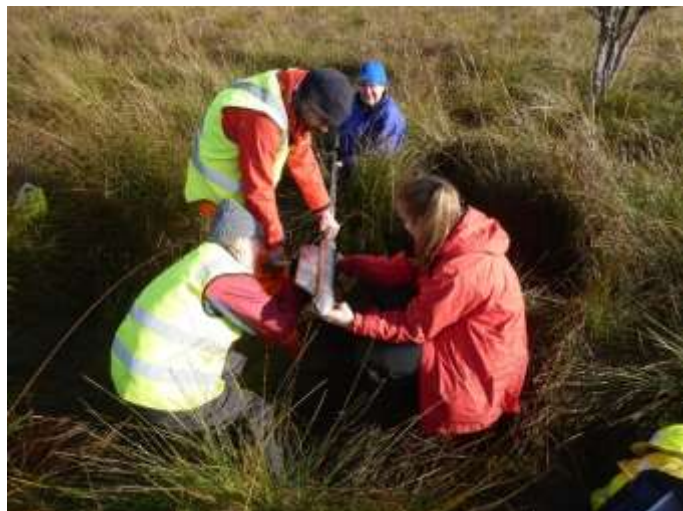
FPA and University of Queensland researchers obtaining a peat core from Yellow Marsh, Surrey Hills.
