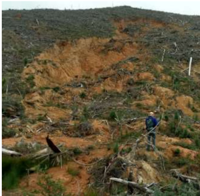
Earth Sciences and Cultural Heritage Program Manager Peter McIntosh surveying the extent of a large complex landslide formed during the June 2016 flood event at Oldina.
