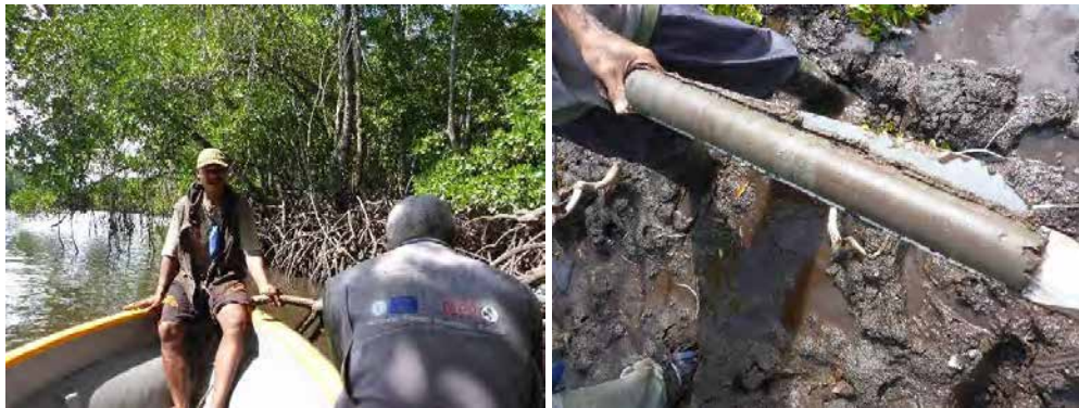
Deep soils accumulating under mangroves can store up to 1000 tonnes of carbon per hectare. Special techniques had to be developed to sample mangrove swamp soils in the Papua New Guinea soil survey (right). These were documented in an FAO report written by the PNG soil survey team with the assistance of the FPA consultant earth scientist.
